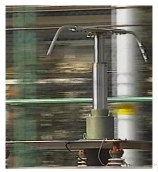
Wingraph power collecting test at RTRI Photo courtesy of Nakatsu, Eiji the-century. The new design comprised two streamlined parts: a pantograph slider (a flattened horizontal foil or wing of copper, iron and aluminum that served as a skid for the overhead live wires), and a aluminum vertical base or pillar, spindle-shaped in cross-section.
