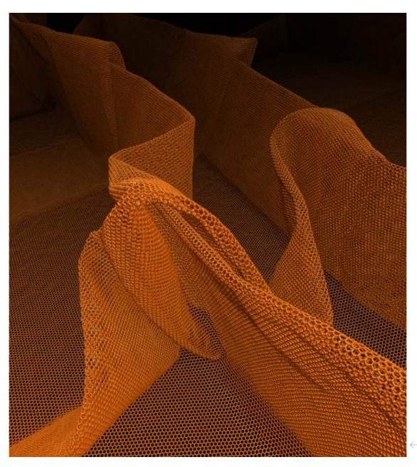
Molecular structure of folded graphene. A synthetic material, graphene can be used effectively to construct complex hierarchical materials. Here, the material is used to mimic the nanostructure at the surface of superhydrophic materials as found in Lotus leaves.
