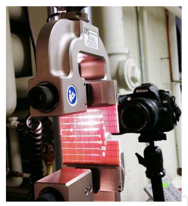
Experimental setup in which the 3D printed composite material is tested under extreme mechanical loading. This setup is used to extract strength and toughness and other mechanical properties of the material. Photo courtesy of Markus J. Buehler and Graham Bratzel (MIT)
