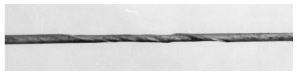
Figure 1. A tube made from helically wound glass fibre in a resin matrix. It has been stretched and has failed by the resin cracking between the fibres
