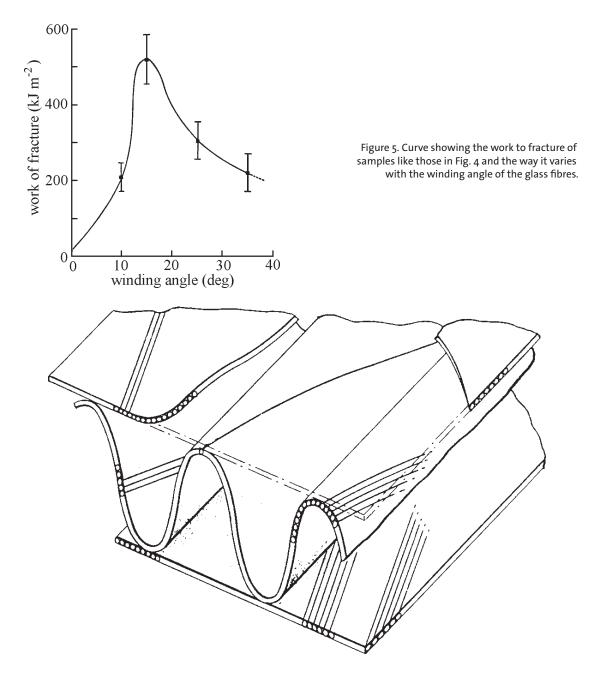
Figure 6. Another version of George's Wood using the technology of corrugated cardboard. The groups of parallel lines indicate the orientation of the fibres in the sheets of pre-preg.
