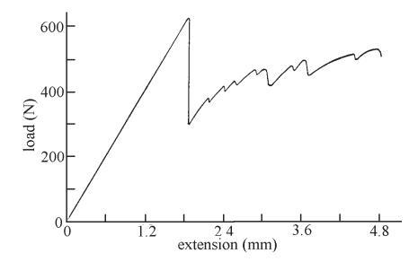
Figure 3. Force deflection curve of a single helically wound tube. The initial failure, followed by a number of minor failures, gives a curve rather like a ductile metal, showing yield and post-yield ductility. But the components from which the tube is made are both brittle.
