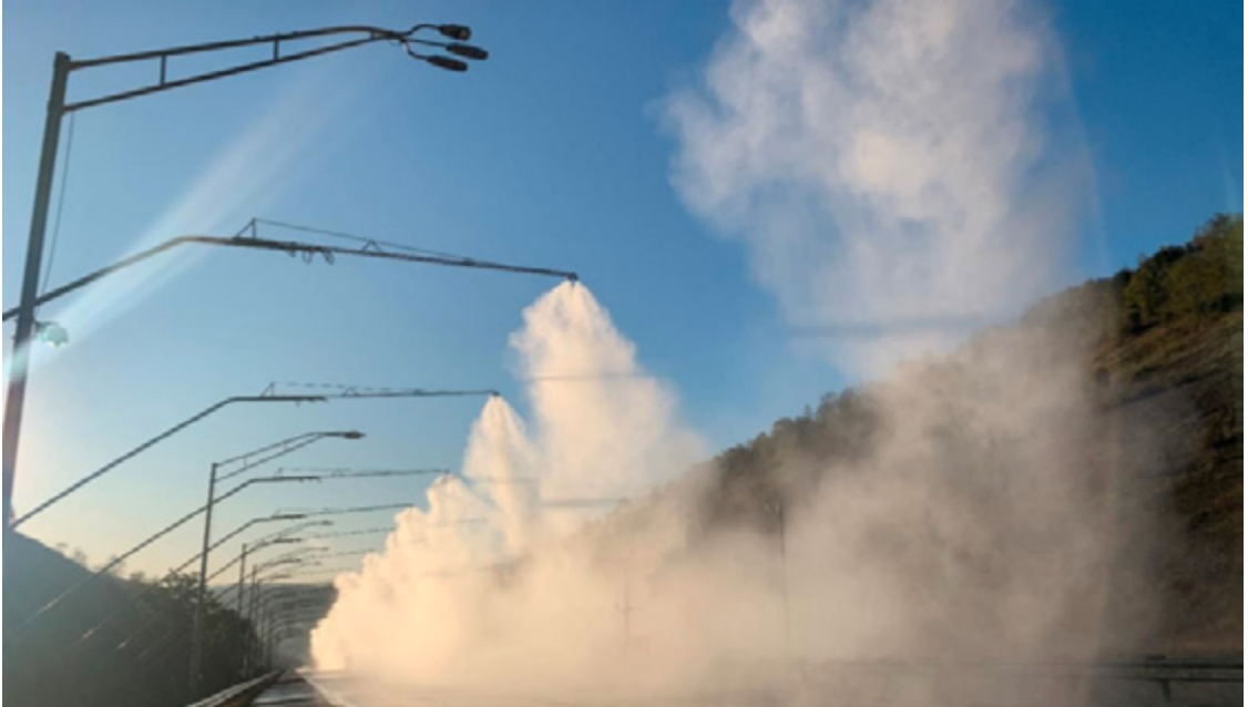
Figure 4a. Fog machines on the Virginia Tech Transportation Institute smart road where controlled round 2 field tests of small fog collectors (SFC's) were performed in October 2019. Bottom: an image of a round 2 Fog Harp under construction using an EDM cut metal comb to keep wires parallel.
