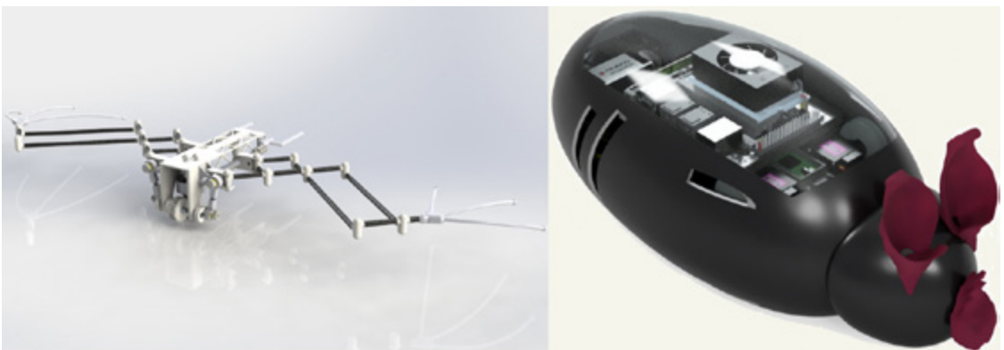
Image 1: Biomimetic robots inspired by bats. a) design that reproduces the flapping flight of bats (Image by Anshool Pradhan), b) biomimetic sonar system with deformable emission ("noseleaf") and reception structures (ears)(Image by Richard Carter).
