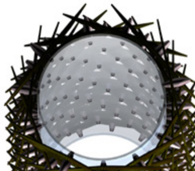
Fig 11. bioTower Anatomy. X-Prize and Inhabitat Biodesign Competition Panels. 2016. (Honorable Mention). Two microbial facade strategies whose data were derived from scanning electron microscope images and CAT scan investigations to inform the design of bioremedial panels tasked to eradicate airborne toxins.
